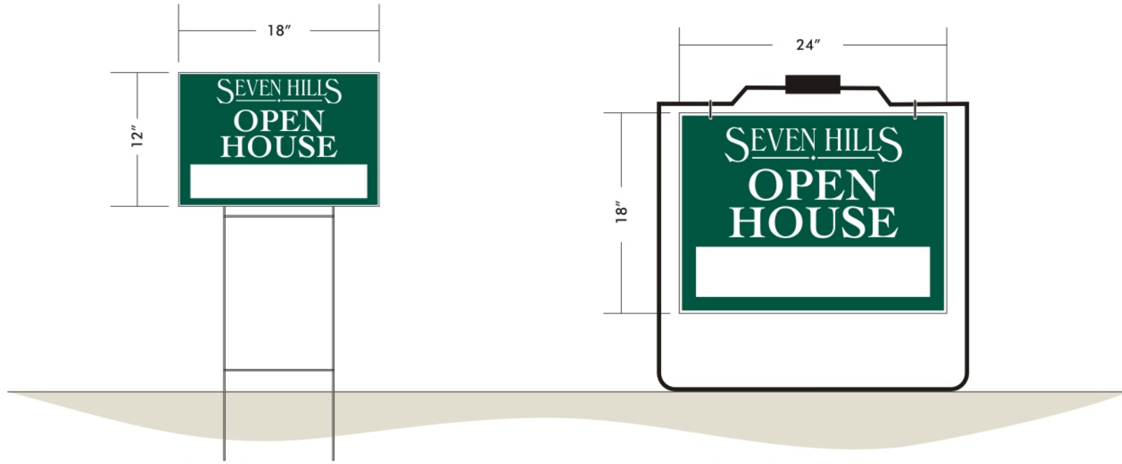
12"x18"x4mm D/F COROPLAST SIGN (VERTICAL FLUTES) W/ VINYL GRAPHICS INSTALLED ON WIRE-H-STAKE BOTH SIDES OF SIGN ARE IDENTICAL
